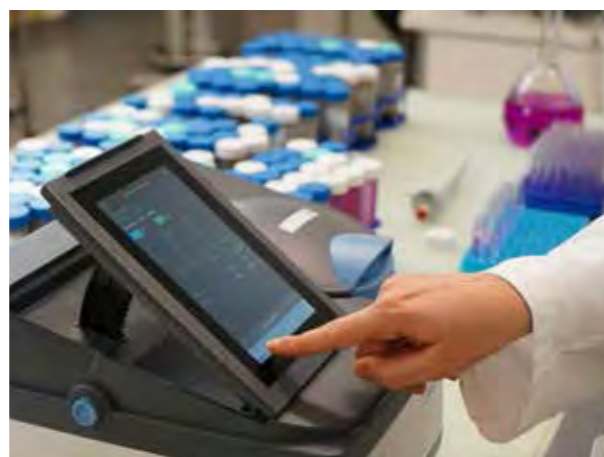
Using a spectrophotometer, Giulia Bongiorno determined the proportion of different types of soil carbon.
